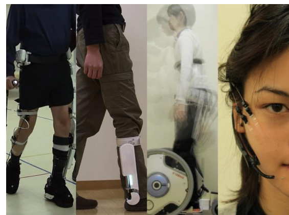
Figure 3. Wearable and assistive robots (from left): Body-synergy based control for exoskeleton [5], ankle-foot orthotic device with the MR-link [8], a standing mobility vehicle with the passive assistive limb [7], and robot mask designed to support rehabilitation of facial paralysis [9].
