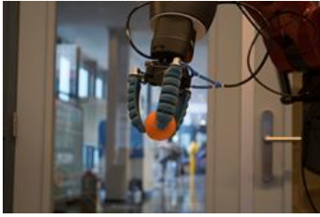
Figure 7. Gripper with multi-material structures that prevent twisting of the fingers.
