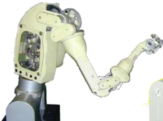
Dexter arm (S.M.) Low size and mass, thanks to cable transmission
