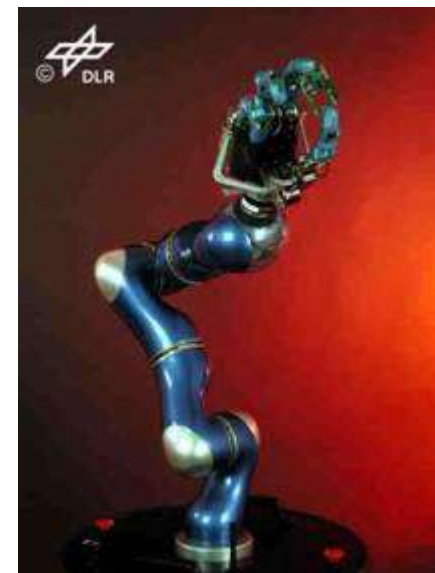
DLR lightweight arm Payload/mass ratio = 1
