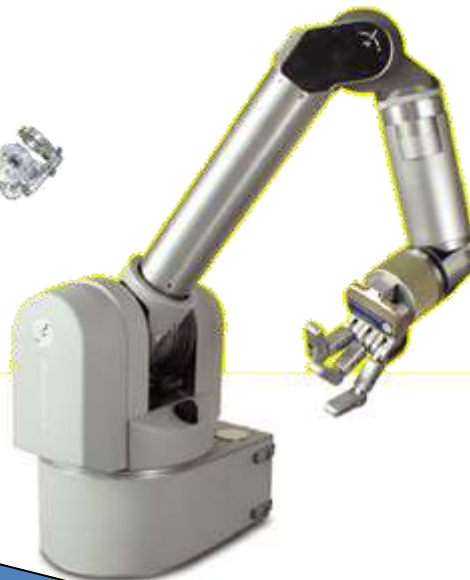
WAM arm (Barrett Technologies) High speed: 20 m/s
