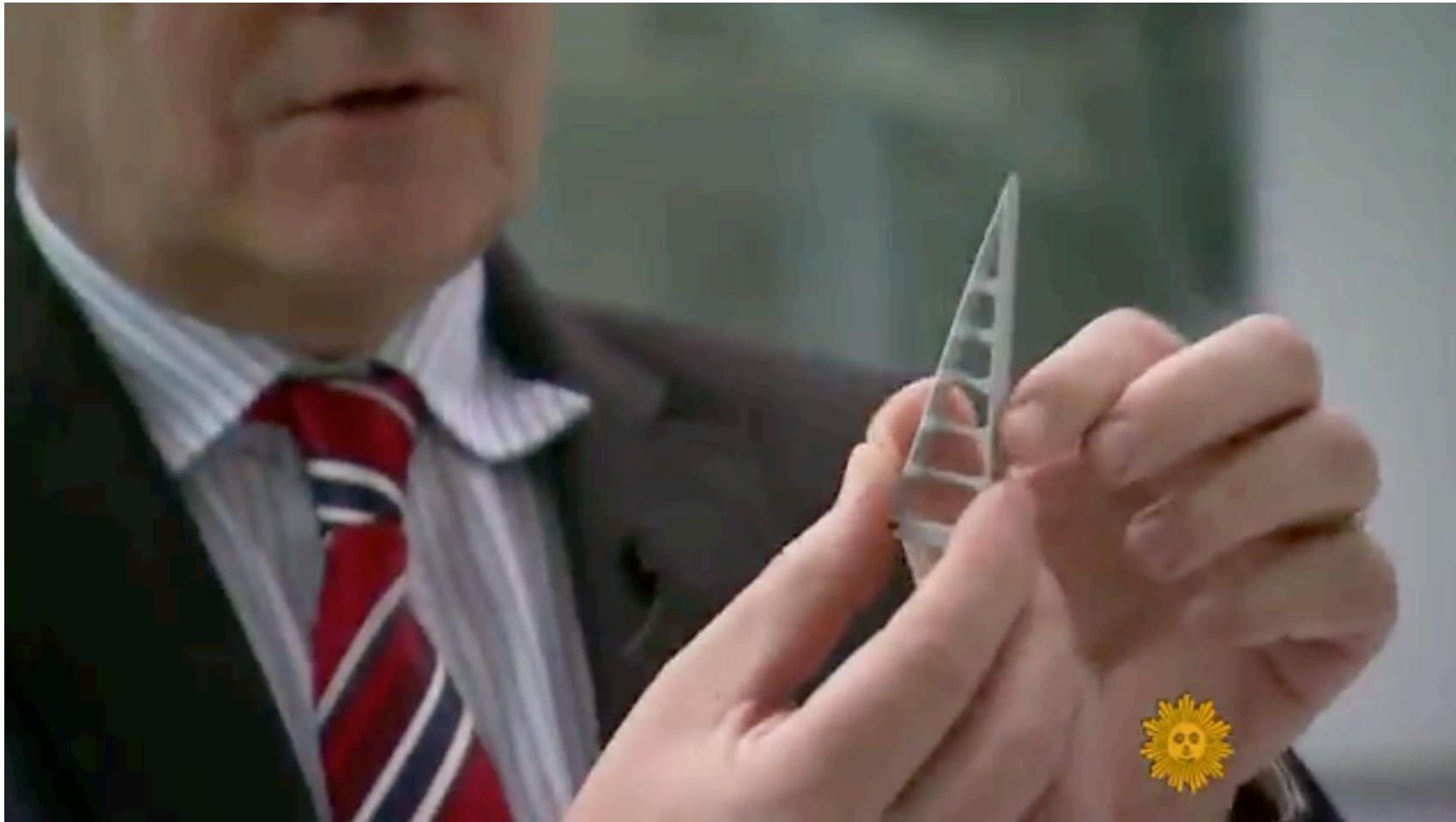
Gripper with deformable materials based on the “Finray” effect
